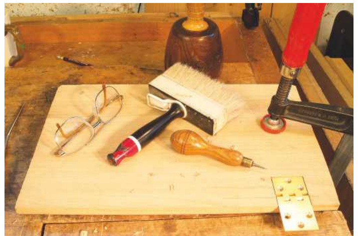
▲ Pic.14 The fitting ready for screws. Note the brush and glasses. It is simple to have a brush handy when chopping accurate recesses in order to remove tiny reluctant chips and Michael finds that wearing a pair of close-up glasses helps avoid costly mis-cutting!
